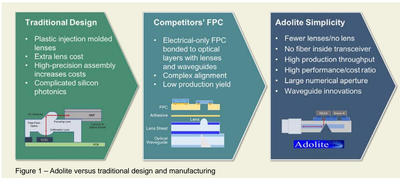
Figure 1 – Adolite versus traditional design and manufacturing
